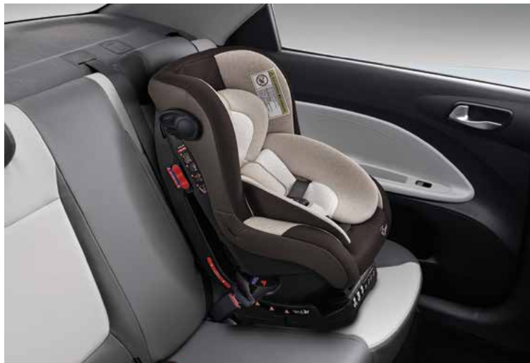
ISOFIX child seat anchors This feature is designed to securely hold child seats for maximum safety.
